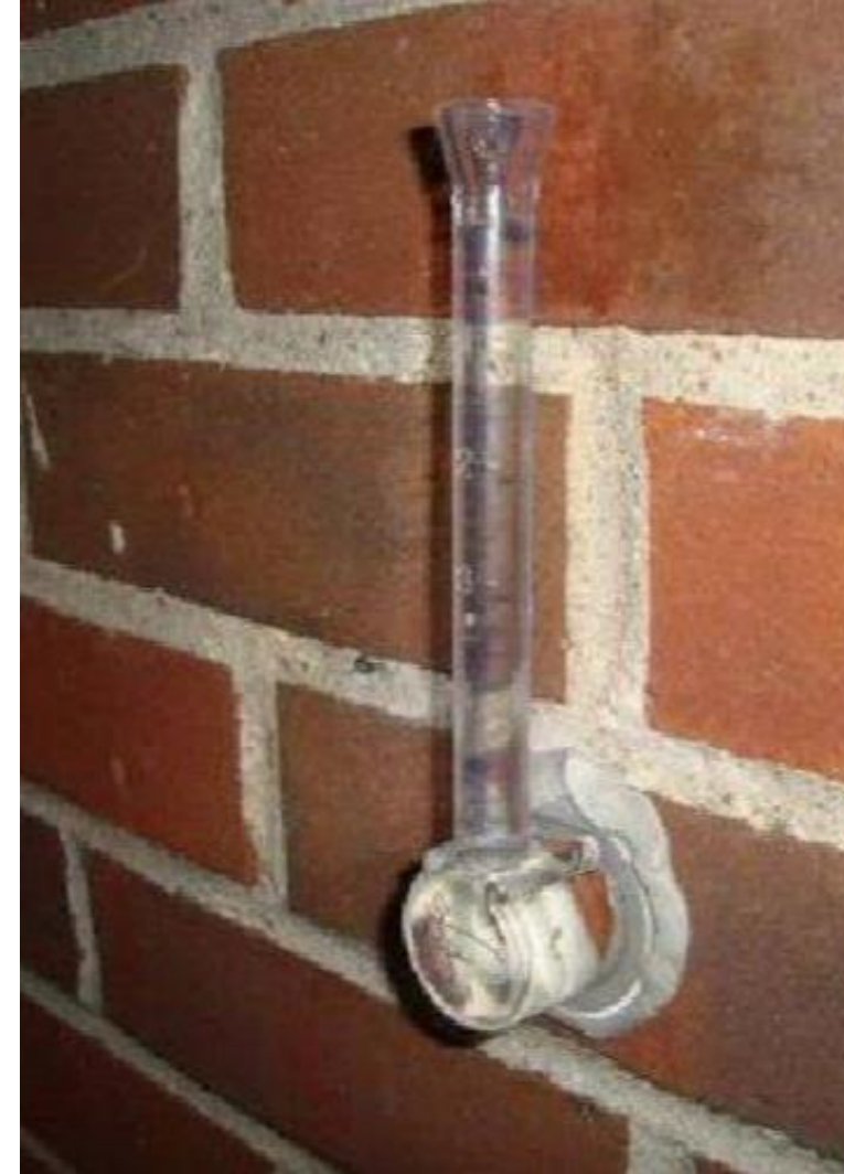
Example of Rilem test in progress
