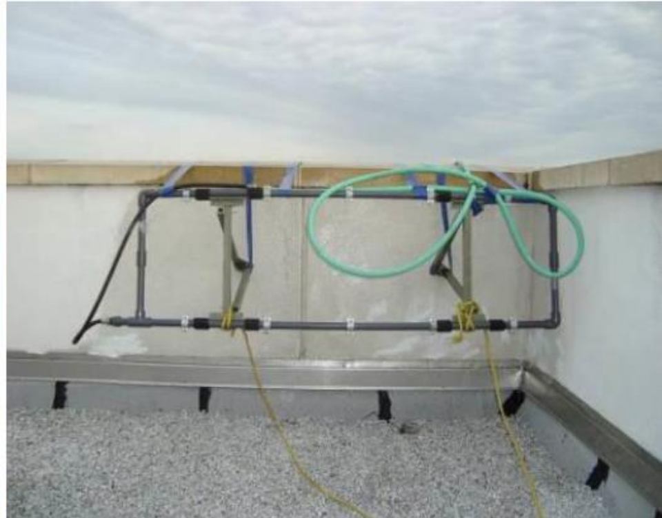
Standard spray testing equipment
