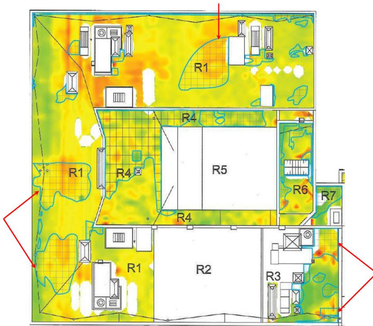
1910 Building Roof Plan, indicating areas of thermal anomalies
