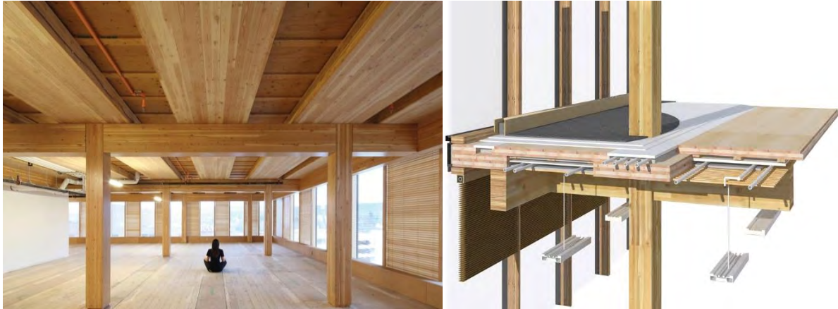
Figure 36. Thickened Floor Plates at the Wood Innovation Design Center, Prince George, British Columbia (Michael Green Architecture)
