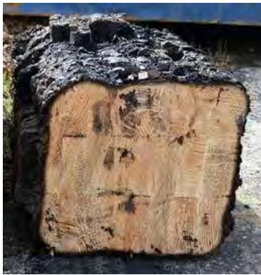
Figure 23. Charring of MT Structural Members (left: ThinkWood; right: WoodWorks)
