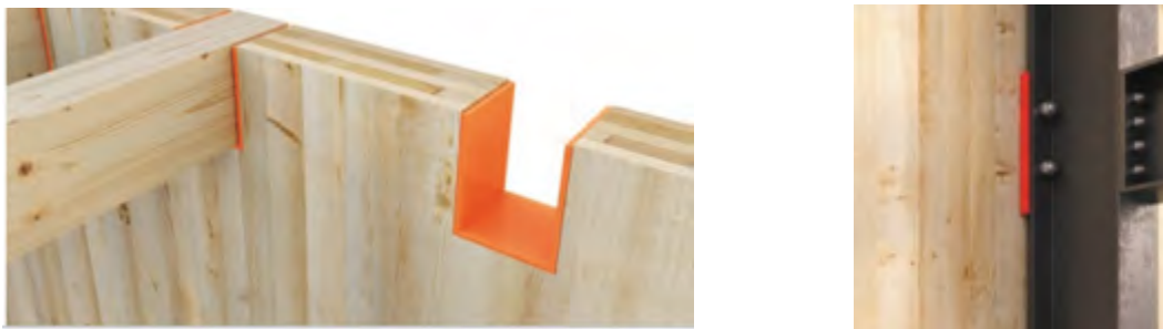
Figure 32. Resilient Pads for Acoustical Separation Between CLT Beams and CLT Wall (left, Woodworks) and Between Steel Column and CLT Wall (right, Woodworks)
