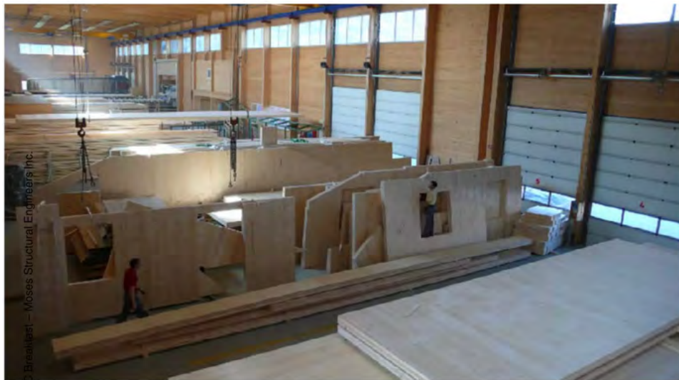
Figure 42. Post-Fabrication Storage of MT Panels By Manufacturer (KLH US Holding Corp.)
