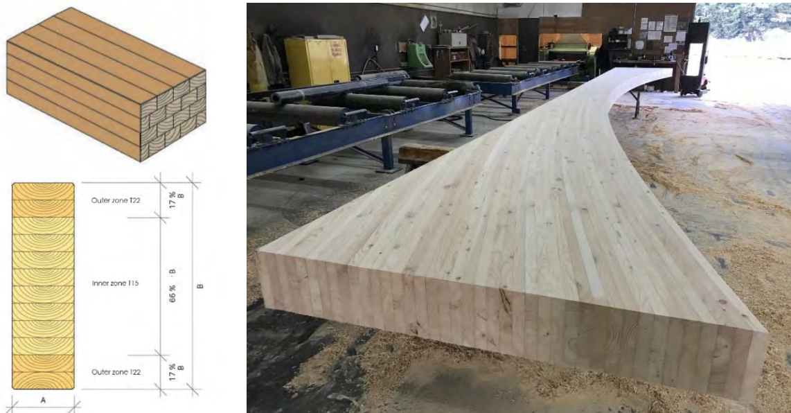
Figure 3. Glue-Laminated Timber: Diagram (top left, Abed et al., 2022) and Layup (bottom left, SwedishWood.com) Curved, Shaped GLT Beam (right, Western Wood Products)
