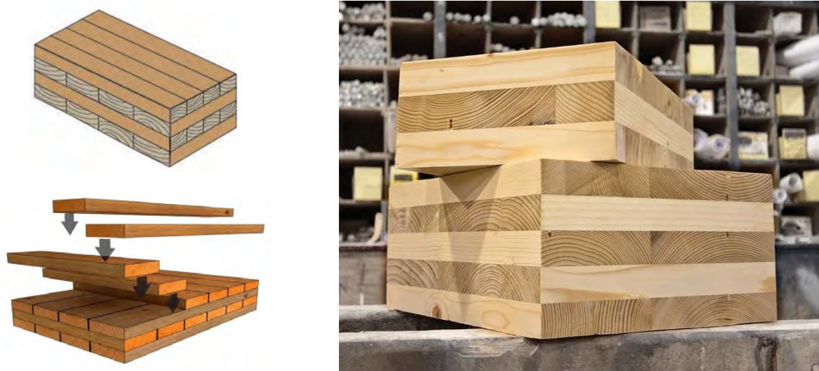
Figure 4. Cross-Laminated Timber: Diagram (top left, Abed et al., 2022) and Assembly (bottom left, Lulea Institute of Technology); Sample Pieces of 3- and 5-Ply CLT Panels (right, Oregon Department of Forestry)
