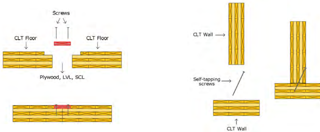
Figure 20. Examples of Wood-Wood Connections (ThinkWood)
