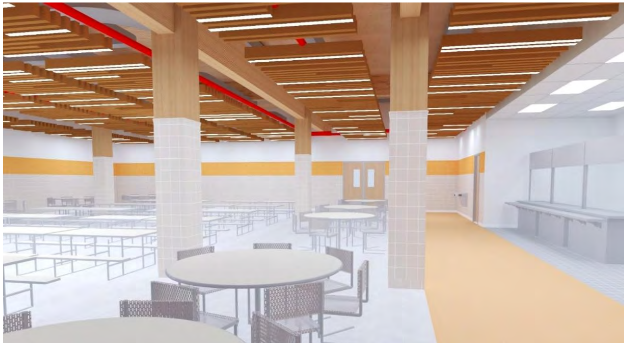
Figure 90. Mass Timber Design - Cafeteria with Wood Baffle Ceiling
