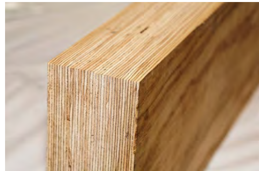
Figure 8. Laminated Veneer Lumber (theconstructor.org)
