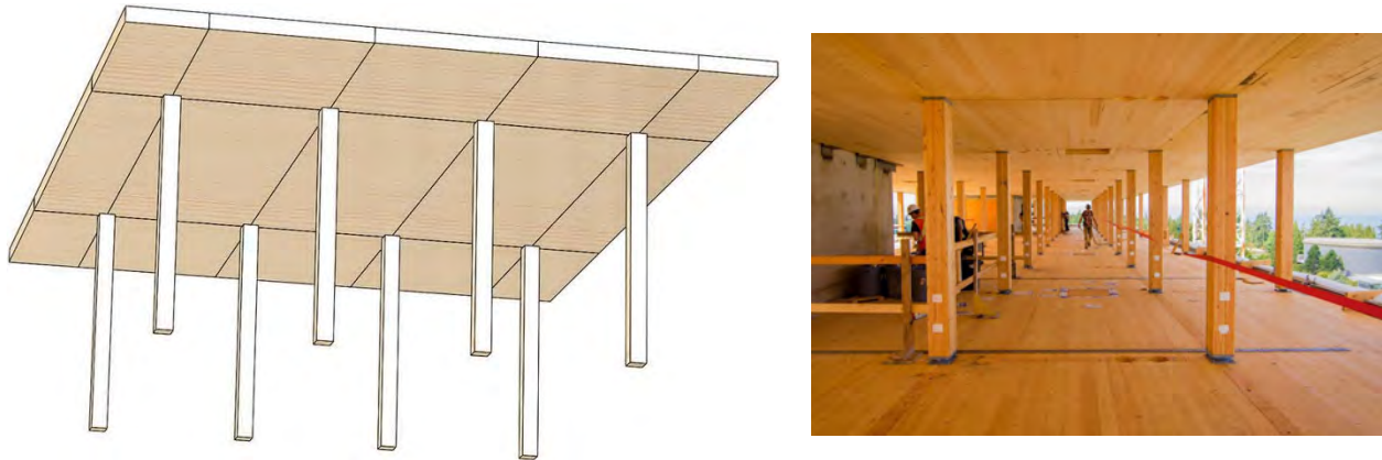
Figure 15. Flat Plate System (left: canadianarchitect.com; right: Acton Ostry Architects)
