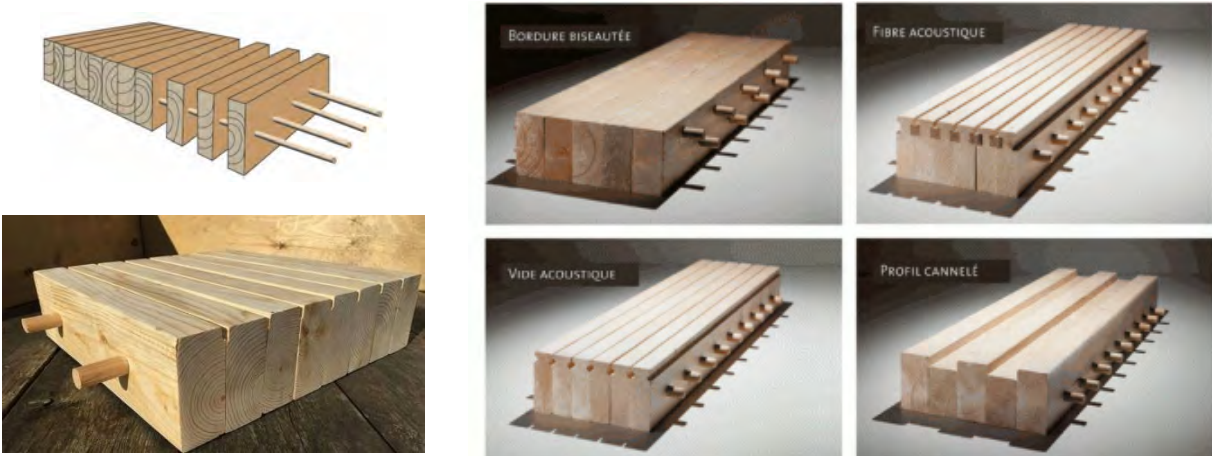
Figure 7. Dowel-Laminated Timber: Diagram (top left, Abed et al., 2022); Sample of DLT Panel (bottom left, Natural Resources Canada); Options for DLT Panel Profiles (right, StructureCraft)
