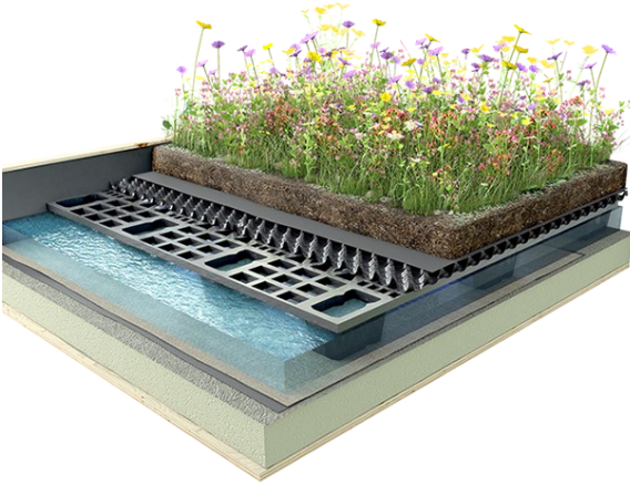
Illustrations of Blue-Green Roof Assemblies (credits: ICB Projects (left), Bauder (right))
